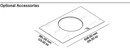
Pre-Construction Bracket (AC-CM6-8EZ-PCB)
