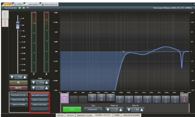
FIGURE 33: The output eq, there are 4 possible alternatives to handle the curve.
